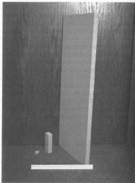
Fig. 9 Foam specimens geometrically similar in two dimensions for tensile fracture test (Divinycell H100)
