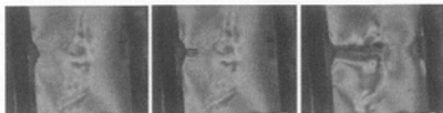
Fig. 15 Development of fracturing compressive kink band at the notch in the laminate skin
