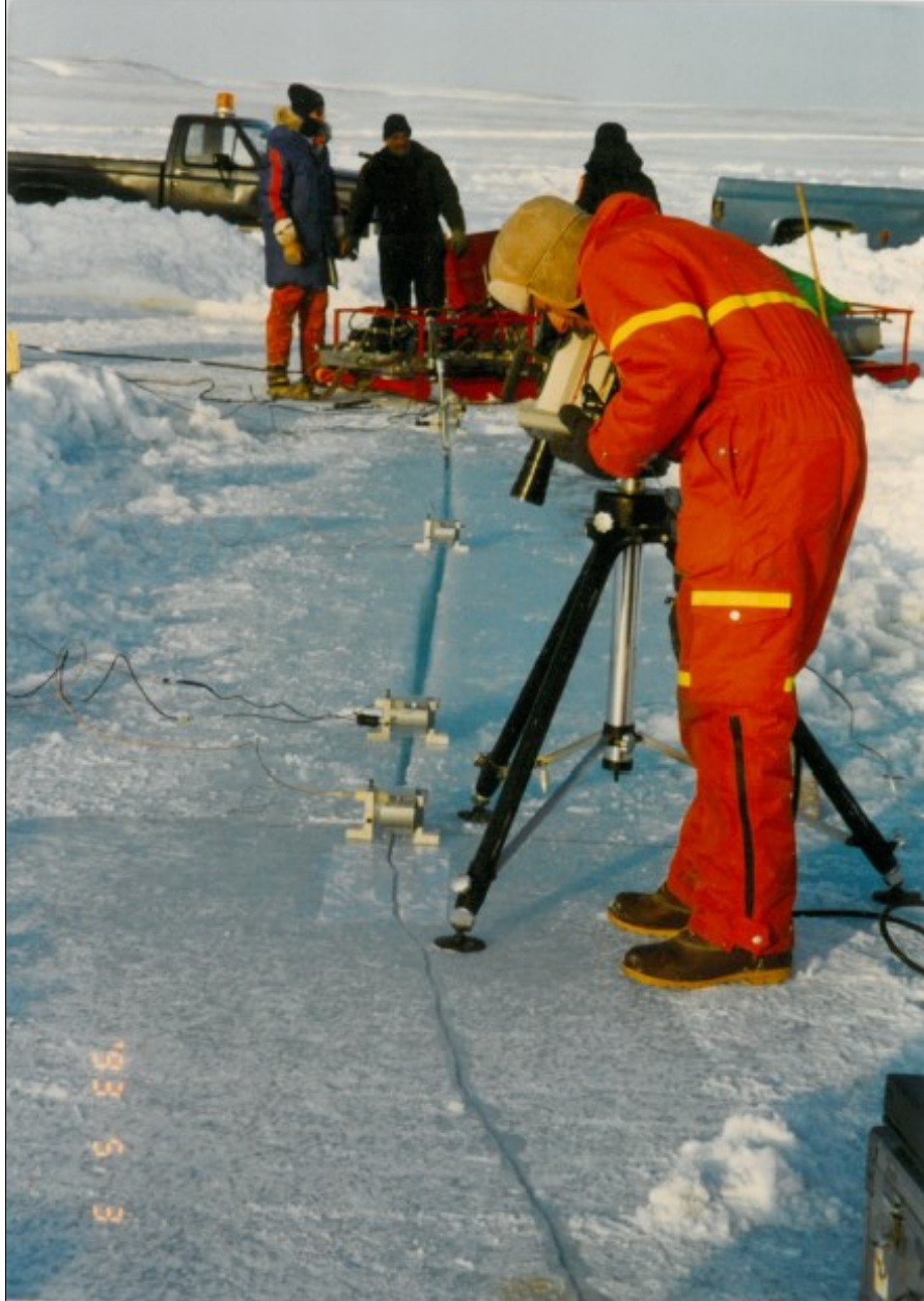
High speed camera recording dynamic crack propagation in scaled-down mid-size specimen. Hydraulic pump assembly seen at distance.
