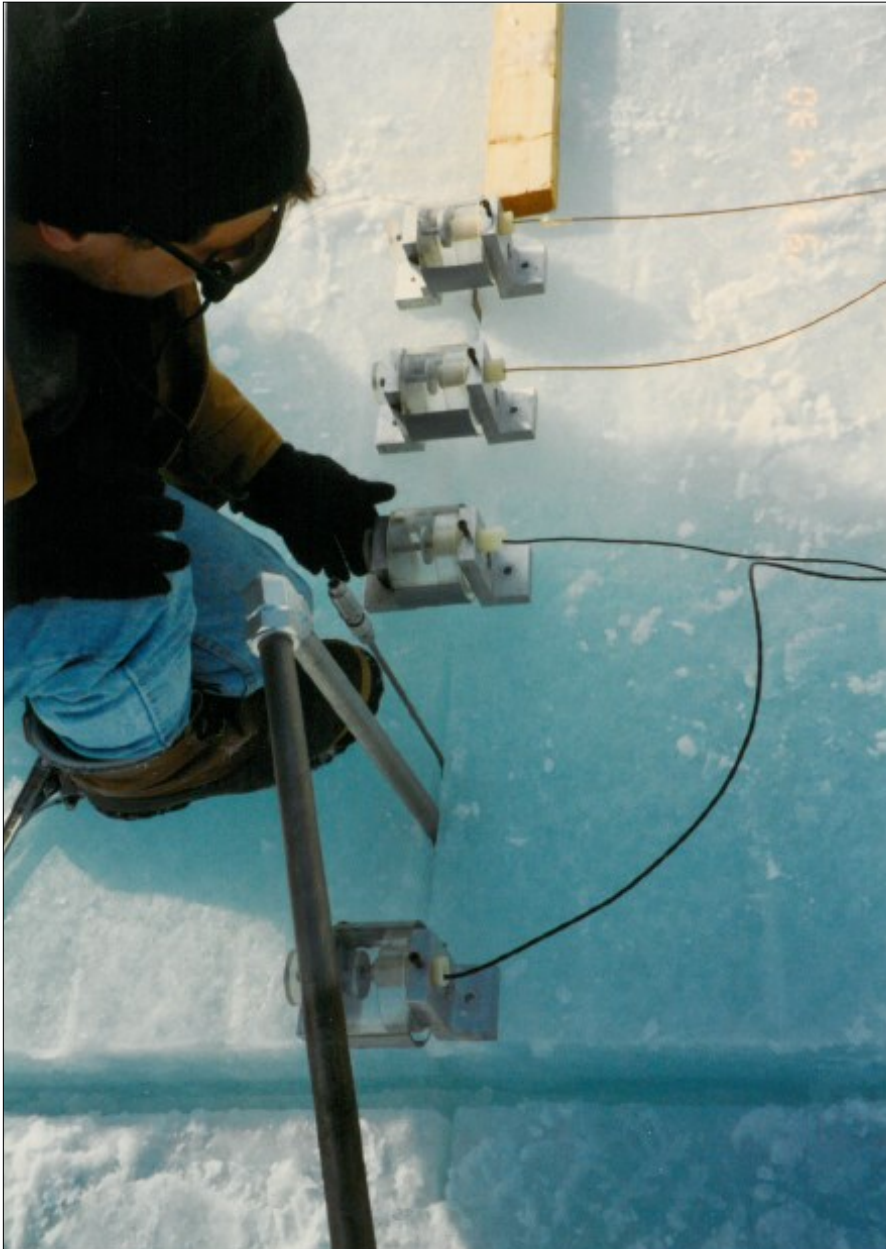
Close-up of crack opening gages from previous photo
