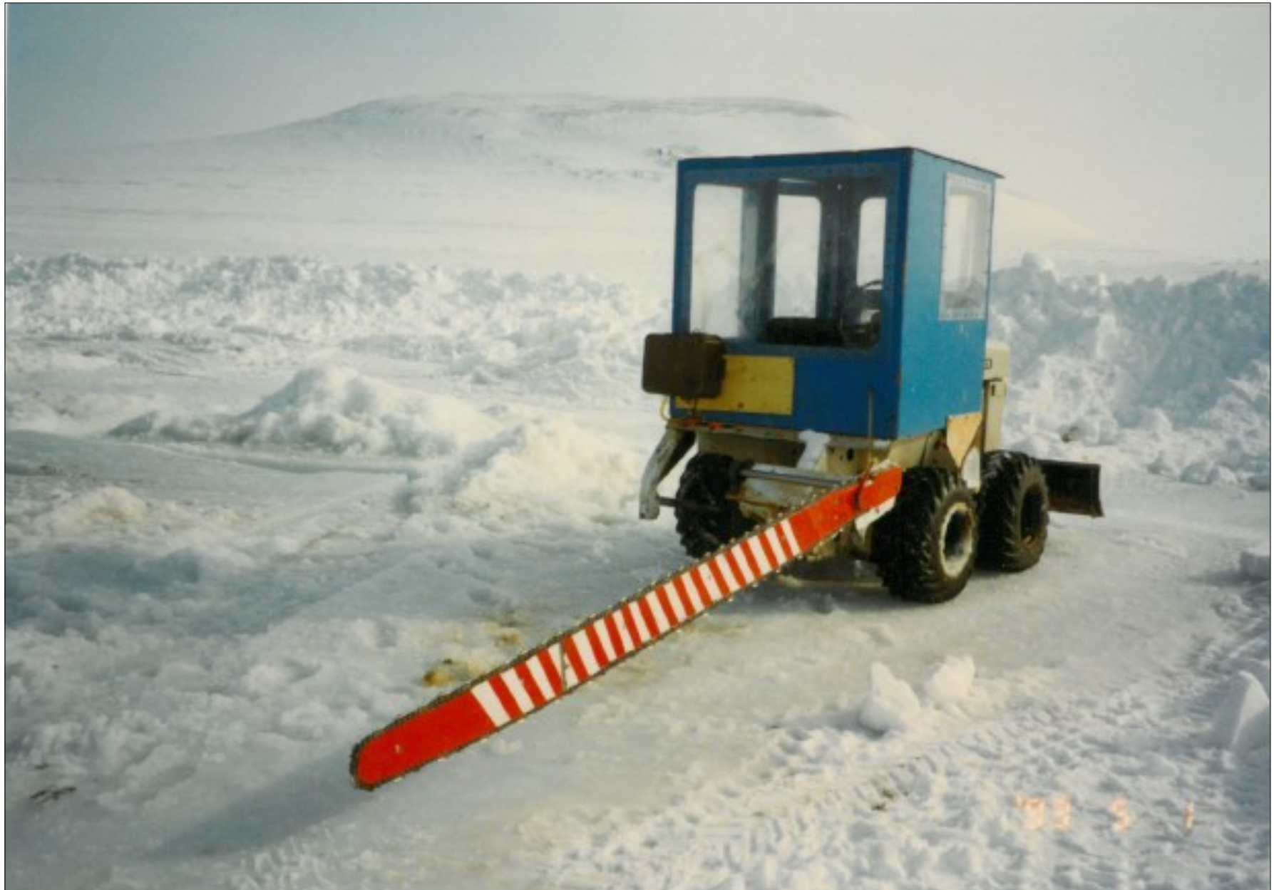
Saw blade for cutting the narrow notch in 1.8 m thick ice (Devon Island in background several miles away)
