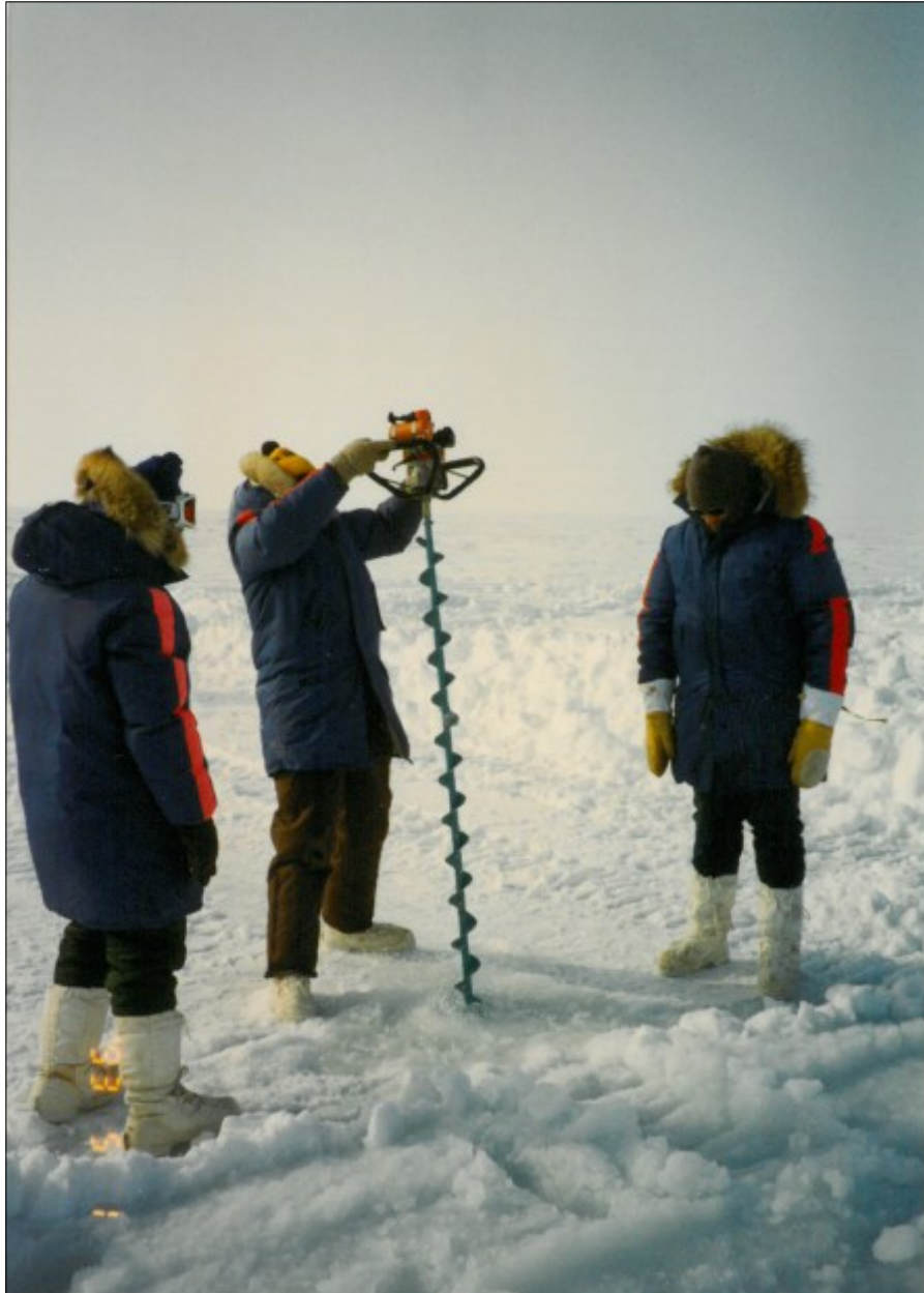
Drill for placing under the acoustic sonars recording dynamic crack propagation.
