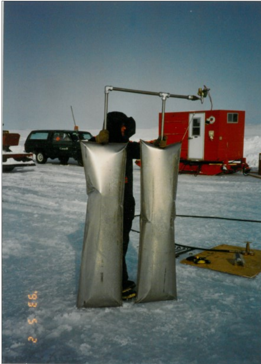
Flat jacks from the largest specimen, pulled out and inflated. Heated computer cabin behind.
