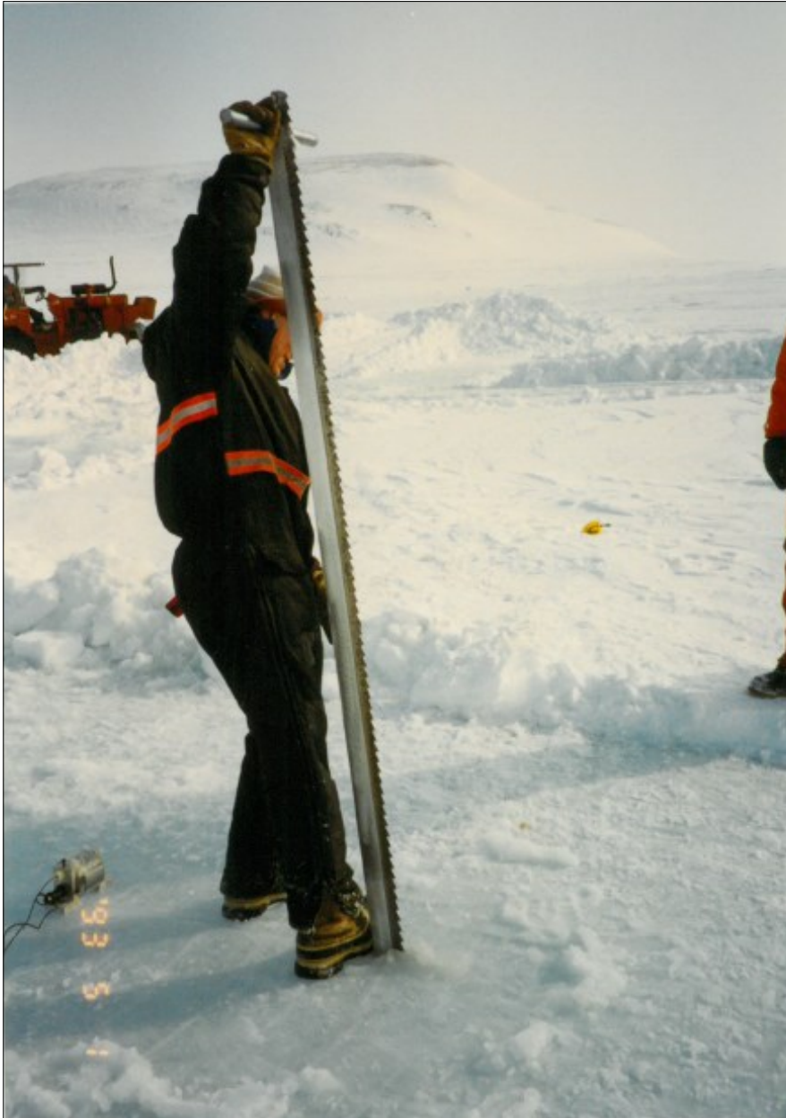
Saw blade for manual sharpening of notch tip (Devon Island far behind).
