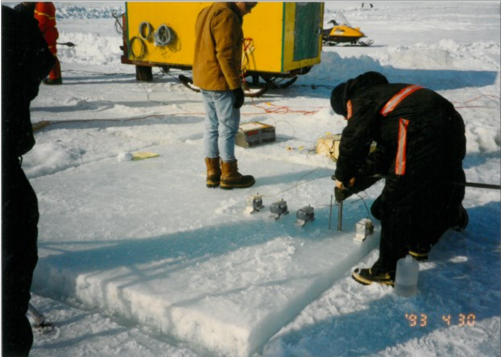
Scaled down 2 m x 2 m specimen, 1.8 m thick, with notch and 4 crack opening gages, and with a pipe extending from a small flat jack. HP computer in cabin behind (the ice was too thick for specimens of side < 2 m. Specimens scaled to sizes down to 0.1 m, but of smaller thicknesses, were tested in a lab on the site).
