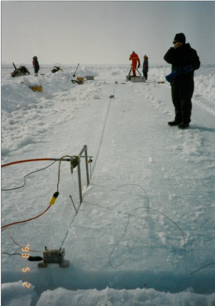
This 24 m long notch cut in the 80 m x 80 m specimen, with pipes of expansive flat jack inserted into the notch. In front: Cayman gage that measures and controls crack mouth opening. 3 more gages a tripod of high speed camera
