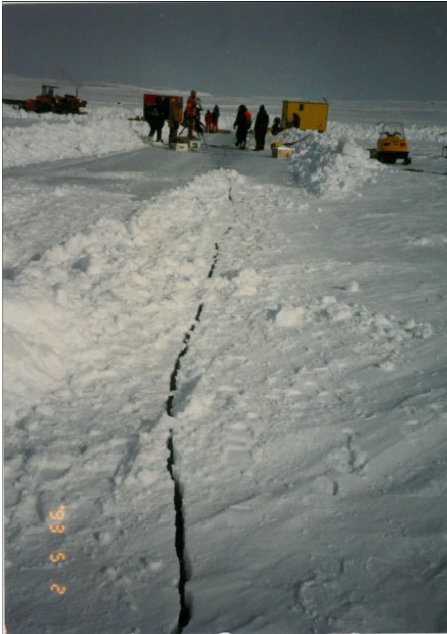
Crack produced in 80 m x 80 m specimen, extending from notch tip in floating first-year ice 1.8 m thick. Computer cabins at distance.
