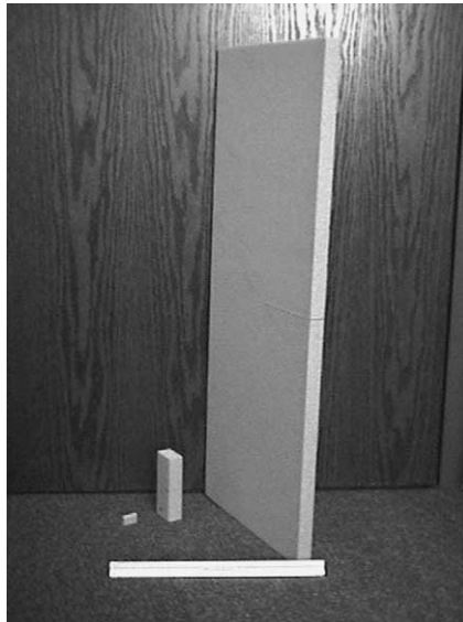
Fig. 1. Foam specimens geometrically similar in two dimensions for tensile fracture test (Divinycell H100).
